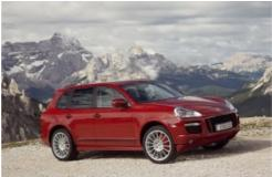
The Cayenne GTS is fitted with Porsche Traction Management (PTM) permanent all-wheel drive and the adaptive PASM chassis as standard. As well as optional air suspension, the Porsche Dynamic Chassis Control (PDCC) active anti-roll system is available to enhance handling and ride comfort. Newly developed 12-way sports seats and a leather-Alcantara mix emphasise the sporty interior.
