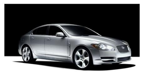
The new Jaguar is likely to maintain the company's recent record of high quality ride and performance, and will be available with a choice of four engines: 2.7-litre V6 turbodiesel, 3.0-litre V6 petrol, 4.2-litre naturally aspirated V8 petrol, and 4.2-litre supercharged V8 petrol (depending on market – the US will only have the V8s to start).
