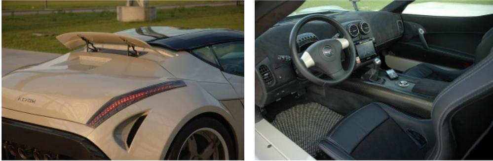
Inside the car, the symmetrical dashboard is characterised by the absence of traditional instrumentation. This has been replaced by a heads-up display projected onto the windscreen, complemented by LED indicator lights and rev-counter on the steering wheel hub. The Sparco seats are carbonfibre, with electric adjustment and memory.
