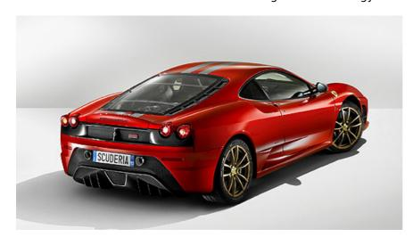
Power from the 4308cc V8 is up to 510 hp at 8500 rpm from the 490 hp of the regular car. This, and the reduction in weight, means the latest F430 variant has an extremely low weight-to-power ratio of just 2.45 kg per hp
