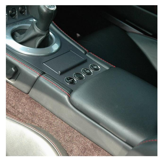
Changes to the exhaust contribute to the gains in power and Prodrive has fitted a driver-operated button to switch between the usual arrangement of valve-opening at 4000rpm heralding the complete V8 barrage, a quiet 'early morning drive through the village' setting where the valve is always closed, and a full-on treatment where the whole world can enjoy your car's performance.
