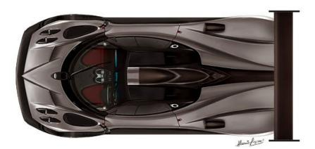
Nor is the car simply an evolution of the Zonda F. It has only 10% of the same components and has been designed from scratch. The wheelbase has grown by 47mm, the overall length by 394mm and the track by 50mm. The suspension forged in Avional, a new Pagani six-speed transverse sequential gearbox, carbonfibre monocoque and aeronautical four-pump fuel tank are just a few of the developments.
