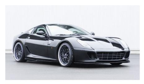
Hamann, the vehicle tuning specialists from Laupheim in Germany, have taken the standard Ferrari 599 GTB and upped the power output of the Enzo-derived 6-litre, V12 engine to give 673bhp. Then they've added some sophisticated aerodynamics and a sports exhaust, made from corrosion-resistant stainless steel, with 90mm tail-pipes - promising an even more awe-inspiring sound than its series production counterpart.
