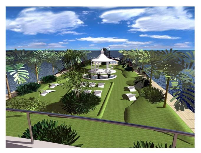
WallyIsland has been designed with a longer length rather than just increasing the height, thus reducing the price and at the same time improving the stability, the result being a sleeker, huge forward deck area of 1,000 m2 (10,764 sq2) that can be devoted to different uses (tennis court, mini soccer court, garden with swimming pool, heli pads...).
