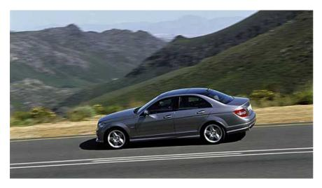
The new saloon is 55 millimetres longer (4581 millimetres) than its predecessor. The body width has increased by 42 mm to 1770 millimetres, and the wheelbase by 45 mm to 2760 millimetres. These dimensions create the conditions for a generously sized interior, and therefore more comfort with front shoulder room increased by 40 millimetres, for example.
