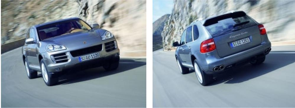
The Cayenne Turbo is fitted with Porsche Active Suspension Management (PASM), with air suspension as standard. This variant can now be augmented with the new Porsche Dynamic Chassis Control (PDCC) roll stabilizer system. This constant roll control, also available for the Cayenne and Cayenne S, limits vehicle roll in corners and counterbalances it completely in most driving situations.
