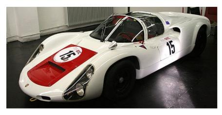
Shorter, quicker and more nimble than its predecessor the 906, the Porsche 910 was first entered in mid-1966, starting with the hill climb from Sierre to Crans-Montana in Switzerland. As engines, either the reliable 2000cc 6-cylinder with 200 hp or the 2200cc 8-cylinder with up to 270 hp were used. The 910 was raced for about two years by the factory, and quite successful during that time.
