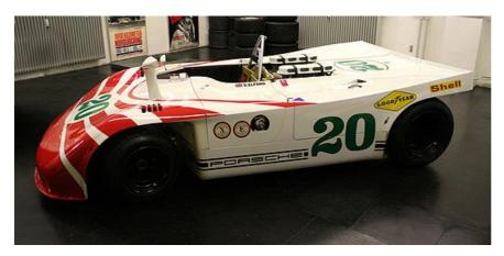
The Porsche 908/3 was designed specifically for the twisty Targa Florio and Nürburgring tracks, where superior handling is essential. The car combined the very light weight of its aluminum-alloy spaceframe and featherlight (a little over 12 kg) glass-fibre bodywork, with a 360 bhp, flat-eight air-cooled motor. In its debut year of 1970, the Porsche 908/3 scored victories in the two races it was designed for; the Targa Florio and the Nürburgring 1000 km.
