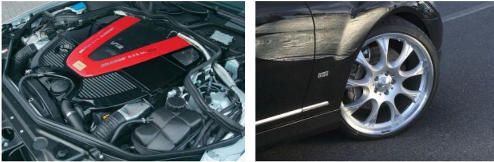
The maximum power output of 730 hp / 537 kW at 5,100 rpm represents a superlative for the BRABUS SV12 S Biturbo engine as does the peak torque of 1,320 Nm at 2,100 rpm. In the vehicle peak torque is limited electronically to 1,100 Nm.
