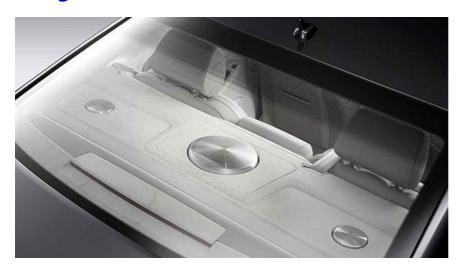
The new Audi R8 will have "...the finest sound system ever fitted to a sports car" says the managing director of Bang & Olufsen Automotive, Jens Peter Zinck. The Bang & Olufsen Sound System has been designed, engineered and developed specially for the Audi R8. It has 12 speakers driven by 10 discrete channels of amplification and digital signal processing, producing a total amplifier power of 465 watts.
