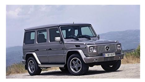
In addition to permanent all-wheel drive with a low-range gearbox, the standard equipment includes the electronic traction system for all-wheel drive 4ETS, the Electronic Stability Program ESP® and differential locks which can be engaged at the touch of a button. Magna Steyr in Graz, Austria, has been producing the G-Class on behalf of Mercedes-Benz since 1979, with more than 186,000 examples built to date.
