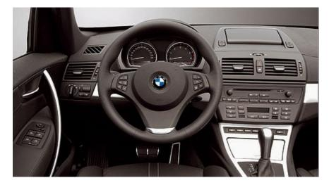
Inside, the driver can get to grips with a new style of three-spoke steering wheel while enhancements to the type of materials used on the centre console have also been included. Again, the owner of a X3 3.0sd gets special treatment with stainless steel foot pedals to underscore the performance nature of the vehicle.
