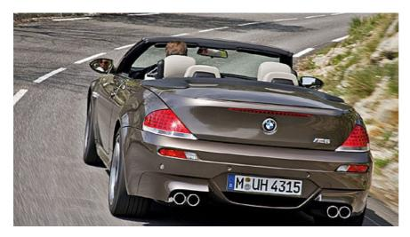
The car features bespoke 19-inch double spoke light alloy wheels shod with low profile performance tyres – 255/40 R19 at the front with 285/35 R19 at the rear. Large vented and drilled high performance brakes
