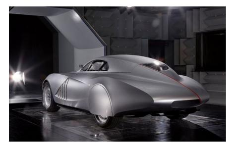
The car benefits from an extremely lightweight chassis. The most modern design processes were used to 'stretch' an aluminium shell over a lattice frame. The body is also constructed from lightweight materials, with carbon-fibre reinforced plastic (CFRP) clothing the entire vehicle, painted in 'fine silver', a full-gloss paint colour with extremely fine pigments that hints to classic silver race colours.
