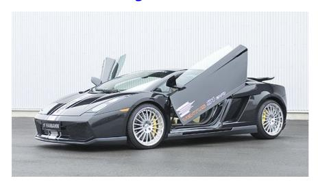
When Lamborghini introduced the Gallardo one of its significant features was, in fact, an 'omission' - the lack of upward-tilting doors in the manner of Lamborghinis past. Now German tuning company Hamann can make your Gallardo truly 'fly', not only via modified aerodynamic components but with the addition of 'gullwing' doors.
