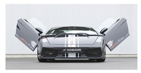
Hamann uses an in-house wing/door construction to create a stable system without being too flashy. The hinges can only just be seen, and don't look retrofitted. This ensures that the Gallardo's driver still cuts a fine figure when getting in and out.
