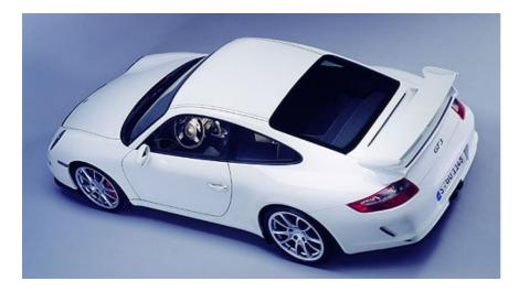
The new 911 GT3 boasts an active chassis for the first time. Porsche Active Suspension Management (PASM) offers two sporty chassis in one: the basic configuration is largely similar to that of the previous model and is suitable for driving on alternating road surfaces. In sport mode, the system switches to harder damping, thereby enabling even better dynamism on the racetrack.
