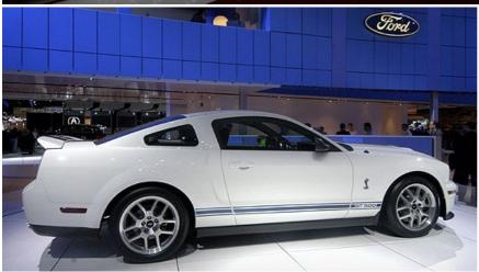
Braking is via four-piston Brembo calipers fitted to 14-inch Brembo vented rotors at the front, and 11.8-inch vented discs in the rear. Tyre sizes are 255/45ZR front and 285/40ZR rear, mounted on  $18" \times 9.5"$  alloys.
