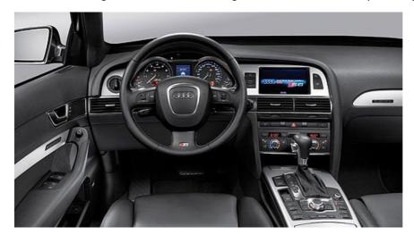
The sporting theme is continued in the facia and doors, which are inlaid with carbon fibre, and in the instrument panel, which features a new 'Flexmetallic' anthracite-coloured metallic covering and incorporates exclusive dials embossed with the S6 logo. Also new within the instrument panel is an upgraded Driver's Information System (DIS) with a built-in digital speedometer.
