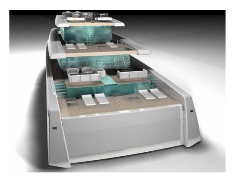
The glass superstructure and the very large portholes flood the interiors with natural light while providing 360 degree view from the upper decks and enhanced visibility from the lower decks. This WallyDesign© project features much larger interior volumes and open air areas than any other mega yacht of the same size.
