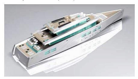
The 55m WallyPower introduces new open air living areas on each deck, especially forward with a superstructure that it is much more ventilated and cooler than aft; where all the other mega-yachts of this size usually concentrate their living areas.
