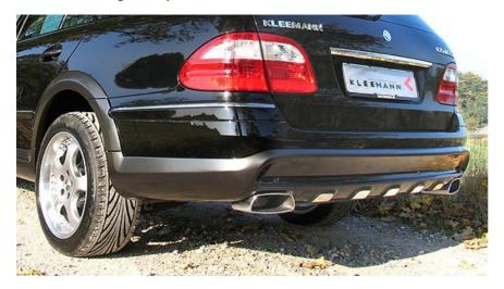
The front and rear skirt, with built-in undercarriage protection in stainless steel, are connected by a bold side skirt and wide wheel arch flares. All together it gives the E50KCC a stern yet sporty look emphasized by polished aluminium roof rails. As usual the rear skirt makes provisions for the trapezoid KLEEMANN exhaust pipes.
