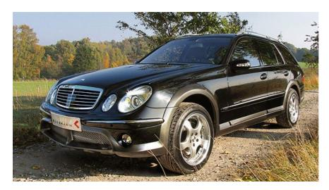
Danish Mercedes Tuners Kleemann believe they have made the perfect car for those wanting an estate car but needing the extra security and surefootedeness of a  $4 \times 4$  in slippery conditions. The E50KCC is based on a regular E500T 4-Matic estate, but has an extra 50mm ground clearance and 595 HP Kompressor V8. The latest Audi off-road version of the A6 is not yet available and this is the nearest thing to it.
