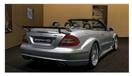
On the outside, the new convertible features a deep-drawn front apron with large air inlets, prominently flared wheel arches, 19" and 20" AMG light-alloy wheels and the diffuser-look rear end with an aerofoil. Numerous body components are made from particularly strong and lightweight carbon fibre reinforced plastic (CRP), for example the bonnet, doors, front wings, flared rear wheel arches and aerofoil.
