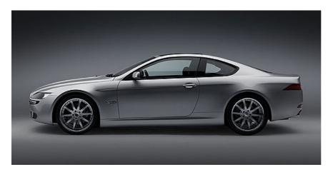
The BMW 6 Series 650Ci Coupe provides the base vehicle architecture for the Fisker LATIGO CS. Final technical details are still being defined, but the standard engine specifications call for a 367 bhp, 32-valve, 4.8-liter V8 - with the V10 from the M6 an option.
