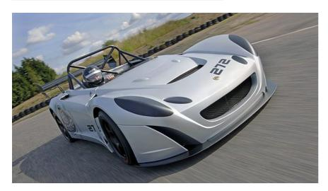
Based on the Lotus Elise Aluminium chassis, and weighing in at approximately 600kg, the singleseater car (with an option of two seats) has been designed and engineered solely for Track Day and Club Racing.
