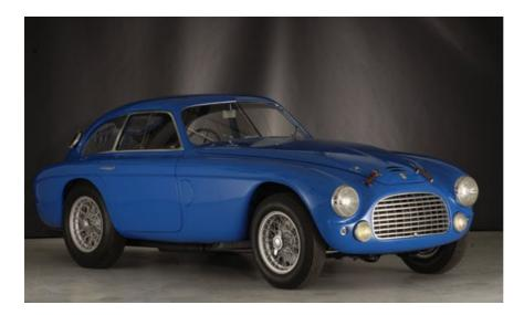
Also entered is another historic Ferrari, the **1950 166MM/195S Le Mans Berlinetta**, chassis # 0060M. Built on the shorter 2,250mm wheelbase, the Touring-bodied Le Mans berlinetta features a 2,341cc V12 specifically built for competition, being rated by the factory at up to 180 horsepower. It had an impressive racing history when new and was the cover car for the Ferrari Club of America magazine, Prancing Horse, in 2002. Estimate: \$1,400,000-1,900,000.
