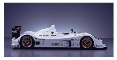
The prototype is powered by a newly-developed 90-degree V8 endurance engine, fitted with ACO regulation air restrictors, delivering around 480 hp from a 3.4-litre capacity. The lightweight power plant features a very low centre of gravity, four valves per cylinder, a dry-sump lubrication system and single cylinder throttle valves.
