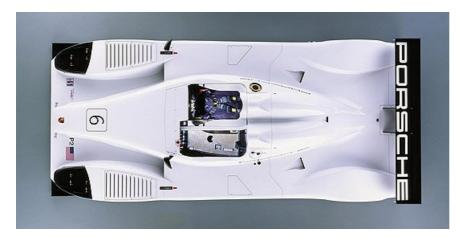
In compliance with the 2006 ALMS regulations, the new Porsche LMP2 weighs in at only 750kg. This minimal weight was achieved through an intelligent, highly integrated lightweight vehicle concept. As the prototype is eventually intended for customer racing, the development engineers had the task of reaching the minimal weight without the extensive use of exotic, and hence expensive, lightweight materials.
