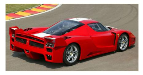
The FXX's aerodynamic design is particularly innovative too as it has resulted in a shape that produces 40% higher downforce than ever achieved before. It is also possible to adjust the FXX's mobile spoiler configuration to suit the specific circuit.
