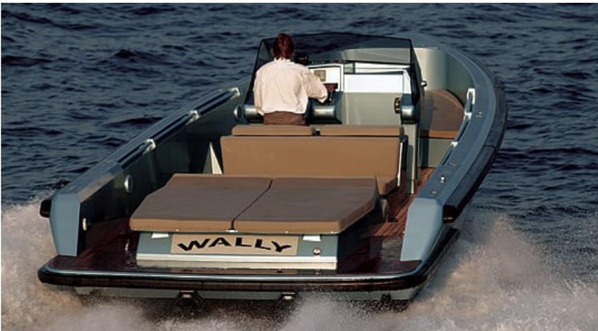
A built in handrail offers safe holding at speed, while the wrap around fender keeps the occupants of the boat comfortably dry when moving quickly; it also provides a practical solution for boarding and docking. The speakers of the hi-fi are integrated with the hull of the boat, and the deck is made of teak that dries out very quickly and is easy to maintain.
