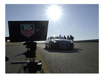
Finally, at the end of April, the technical inspection of the Exelero was carried out on the DaimlerChrysler test track in Papenburg, i.e. the test measurements conducted provided the basis for preparations for the attempt at the high speed record in Nardo. For example, spoilers were tried out in various positions and further adjustments made to optimize the speed and stability.
