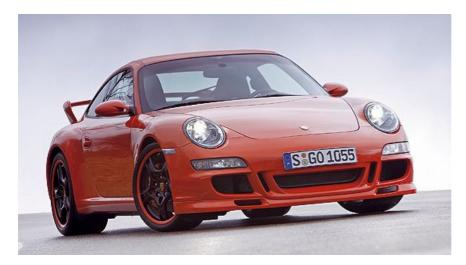
Porsche AG, Stuttgart, now offers a new customisation package for the Coupé versions of the 911 Carrera and the 911 Carrera S. The "Aerokit Cup" consists of a front bumper with an integrated spoiler and a rear lid featuring a spoiler and a rigidly mounted biplane rear wing.
