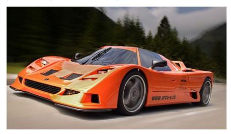
The MTM-optimised AUDI V8 engine produces 650bhp and coupling that with a weight of only 850kgs means the car can reach 100 km/h from standstill in under 3 seconds, 200 km/h achieved in only another 8.5 seconds. Maximum speed is beyond 360 km/h - enough to catch the fastest fish in the world.
