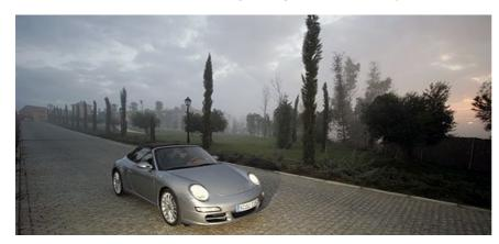
Even top-down, the new car will look after its passengers with the aid of draught-reducing, electrically-operated rear wind-deflectors. The maximum speed of 274 km/h speaks for itself, and lowering the roof takes just 20 seconds from pushing one button. It can also be done at road speeds up to 50 km/h, or remotely via a key when parked.
