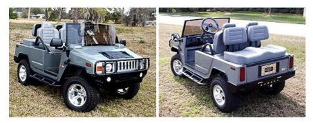
Custom-made bodies are attached to regular modern chassis made by the likes of Club Car, EZ-Go or Yamaha. Further detailed accessories such as leather seats, bumpers and lights are then added. The customer can specify individual colours and finishes – just like on the real car. There's also the possibility of adding some monster low-profile wheels and tyres, as preferred by the baddest dudes in town.
