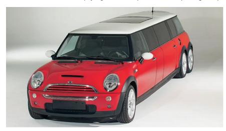
To accommodate the extra body length of the MINI XXL, the car is supported by a third rear axle that has two additional wheels.
