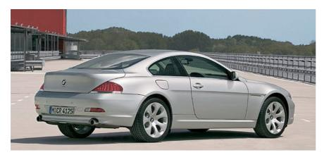
Available in both Coupé and Convertible guises from launch, the 630i develops 258bhp at 6,600rpm, increased by 12 per cent compared to the current 3.0-litre petrol unit. Maximum torque is 300Nm and this is available from just 2,500rpm up to 4,000rpm with the redline starting at a heady 7,000rpm.
