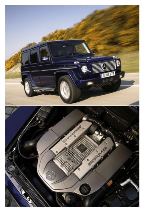
New G 55 AMG with 350-kW/476-hp supercharged V8 engine
