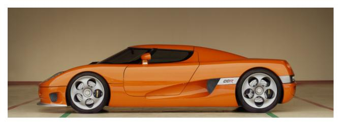
The new model CCR is the top version of Koenigsegg. It has all the features of the CC8S model but a refined design of the side air intakes, different headlight arrangement, a revised rear design, larger brakes, a more powerful engine and small performance enhancing modifications as well as new front splitters for optimized downforce.
