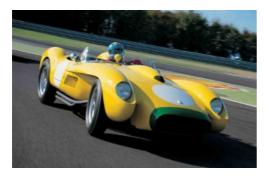
0738 is here at Maranello right back where it was born 45 years ago, still with its original steel chassis, engine, gearbox, axle and running gear. Let's look at some numbers: a 3.0-litre V12 (73mm
