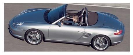
True roadster character is emphasized by lowering the body by 10 millimeters and by especially sporty suspension settings. This sports suspension improves the car's roadholding still further and permits higher lateral acceleration values. Porsche Stability Management (PSM) is installed as a standard feature on this
