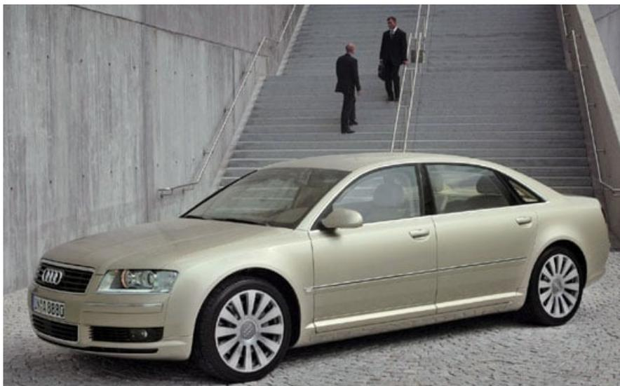
**New A8 models featuring 3.0-litre six-cylinder petrol and TDI engines make their international débuts at the 2003 Frankfurt Show. The Common rail 3.0-litre TDI creates the first ever EU4-compliant and the 3.0-litre petrol model is the world's first luxury saloon to feature Continuously Variable Transmission (CVT), maximising performance and fuel economy**
