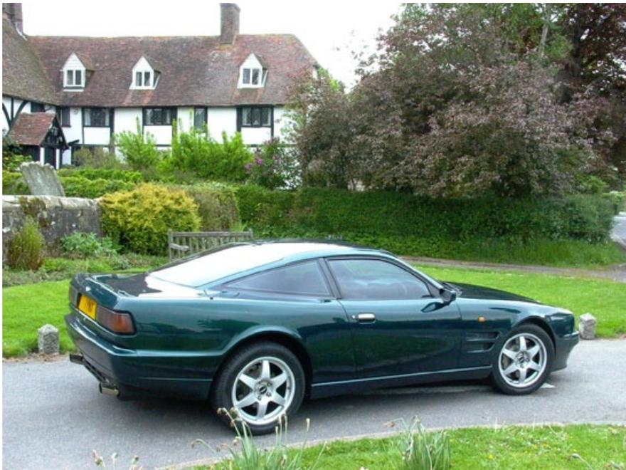
**Built by Lynx in 2002, this highly modified Virage is now powered by a 7 litre turbo charged version of the original 5.3 litre unit. Power output is 725 BHP at 4,000 rpm with a peak torque of 1,150 lb/ft at 3,100 rpm.**
