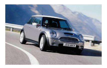
A 163bhp, supercharged MINI Cooper S will be on sale from June, at an on-the-road price of £14,500. The S uses the same 1.6-litre, 4-cylinder transverse engine as existing MINI models, but breaks the "magical" 100bhp per litre figure through the use of supercharger and intercooler technology. Complementing the uprated engine is a new six-speed gearbox.
