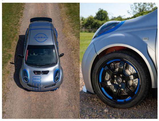
Powered by a mid-mounted 3.5-litre V6 from a Murano upgraded with headers from a 350Z, NISMO high-lift cams and induction, plus a modified ECU, this 1,200kg hot hatch has been endowed with over 300 horsepower. For years now, the Micra 350SR has brought smiles to the faces of Nissan event attendees and journalists alike, and now they're honouring its service with a restomod-style refresh.
