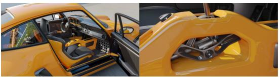
In order to endow the Carrera Coupe with handling to match its poster-car looks, Singer has equipped their latest reimagined 911 with new, four-way adjustable dampers featuring electronic driver-adjustable damping control and a nose lift system. Meanwhile, for maximum stopping power, customers can specify carbon ceramic brakes developed through Singer's DLS services, which fit neatly behind the model's 18-inch centre-lock wheels.
