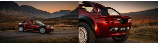
With a bespoke suspension system, offering increased ride height and width while refining the body control to inspire confidence, the Elise takes on a new lease of life, and one that include dirt tracks as well as the open road. A new powertrain also delivers strong, reliable performance, while key functional upgrades - including a limited-slip differential, and a hydraulic handbrake - contribute to the car's uniquely playful character.
