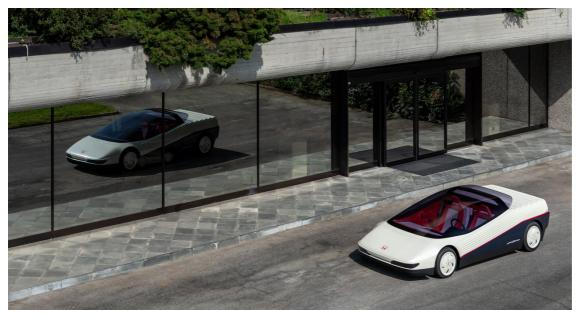
Above all the tech, however, the HP-X's most striking feature has to be its single-piece perspex canopy, which eliminated the need for doors. Climb inside, and you'll notice the HP-X employed many now-commonplace features such as GPS, real-time telemetry, and even a special sonar system that provided road condition warnings. We can't wait to see this ambitious concept on the concours lawns later this month!
