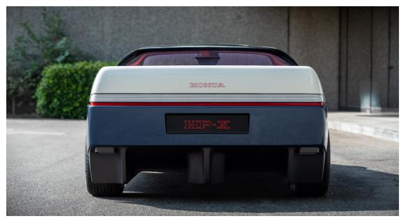
While it's hard to believe this is a design from the 1980s, the HP-X preceded the development of the NSX and was built to show Honda's intent to bring a mid-engine supercar to market. It featured cutting-edge technology, such as ground effect aerodynamics, carbon fibre and Kevlar construction, and innovative cooling methods for its Honda F2 racing engine-derived 2-litre DOHC 24-valve V6.
