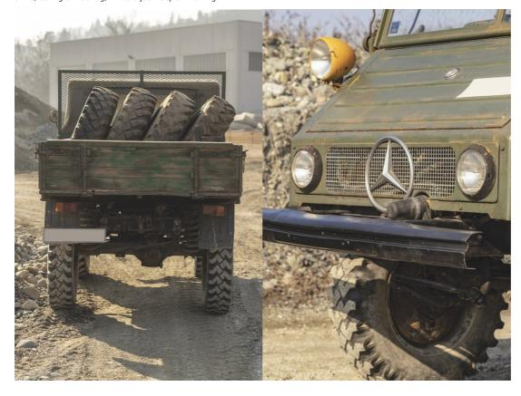
After initial production in 1948, Mercedes-Benz took over the assembly line three years later, and produced a much larger density of Unimogs with many different industries in mind. These vehicles were void of any of the renowned Merc luxury, but they more than made up for it with their ability, featuring an ingenious flexible chassis design that allowed this giant vehicle to scale even the toughest of terrain.
