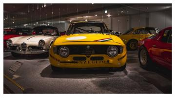
This particular GTA is a Group 5 'semi-works' Monzeglio example with the more aggressive FRP fenders, bonnet, boot, and doors. Between 1968 and 1972, 447 1300 GTAs were made. 300 of those were Corsa versions, intended to race in and dominate the touring-car classes of the time.
